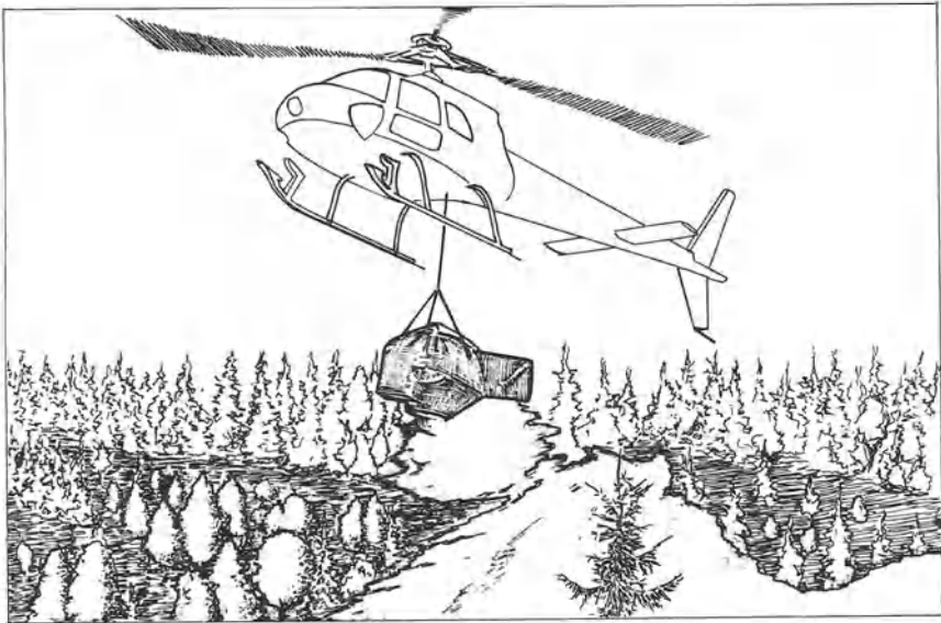
Figure 5. Helicopters are commonly used for liming of poorly accessible lakes. Drawing by J. Wohlke.
